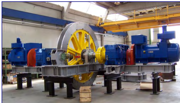
The main winch: pre-assembling in Agudio factory.
